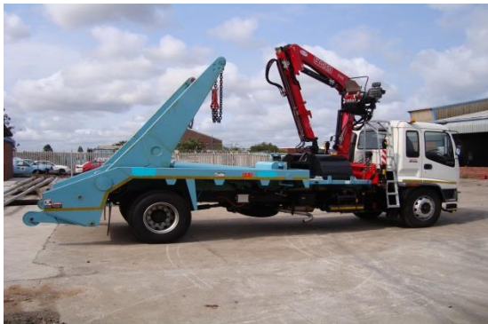
Picture above: Configured skip truck with crane..
